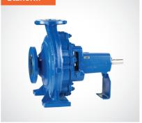
Horizontal, end suction, centrifugal, radially split volute casing pumps in back-pull-out design fitted with single stage radial impeller.
