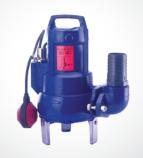
Vertical, monobloc pumpset, free flow impeller of two sizes, 1Ø and 3Ø motors with IP 68 protection, 1Ø motor with built-in thermal overload protection and float switch, bi-directional mechanical seal
