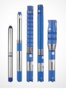
Submersible pump in multi-stage construction with radial or mixed flow impellers coupled with oil or water filled, single or three phase submersible motors.
