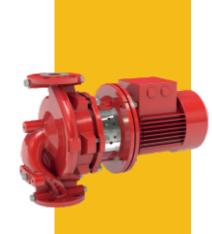
Single stage inline volute casing pumps with back pull out design and ratings to EN 733 with radically split volute casing replaceable wear rings, stub shaft design. Closed radial impeller, single mechanical seal to EN 12756 and a shaft
